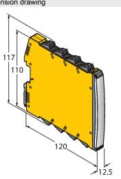
Isolating switching amplifier, 2-channel; SIL2 acc. to IEC 61508; Ex-proof version; 2 transistor outputs; input Namur signal; ON/OFF switchable monitoring of wire-break and short-circuit; toggle between NO/NC mode; signal doubling; removable screw terminals; 12.5 mm wide; 24 VDC power supply
