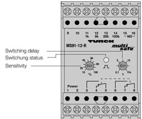
The 1-channel level control MS91-12-R monitors and regulates conductive liquid levels (II). As a dual level regulator, it can be used to control pumps and solenoid valves (I). As monitoring device it is designed for run-dry or over flow protection.
