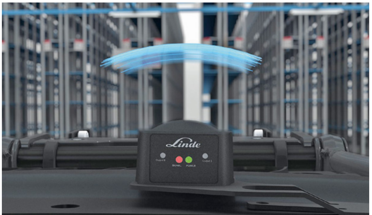
The compact dimensions, robust design and flexibility were key factors in choosing Banner's QT50 as the SpeedAssist sensor, which was manufactured for Linde as a brand label product
