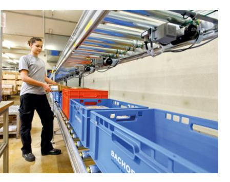
In applications using many read/write heads, wiring effort is reduced by the possible cascading of the RFID interfaces devices. During operation the web browser is ideally suited for the diagnostics and maintenance of the connected components and system data. All that is needed is the installation of an HTML5-capable browser on the device. Although the "S" of TBEN-S actually stands for "small" – it could also stand for "simple" on the TBEN-S-2RFID-4DXP.
