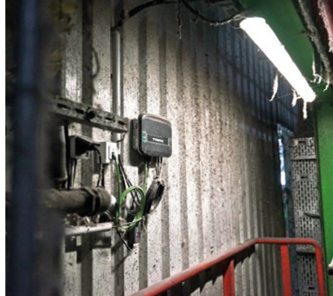
Thanks to its high IP67 protection rating, TURCK's robust Q180 RFID reader performs reliably even in the harshest environments
