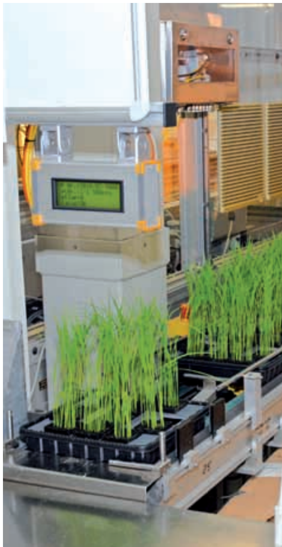
After the plants have passed through the current program, the data can be read on the display
