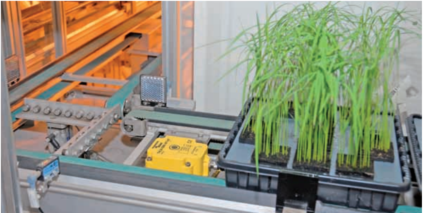
After the plant pots leave the spray units, all the relevant data is written onto the RFID tag in the middle of the plant pot
