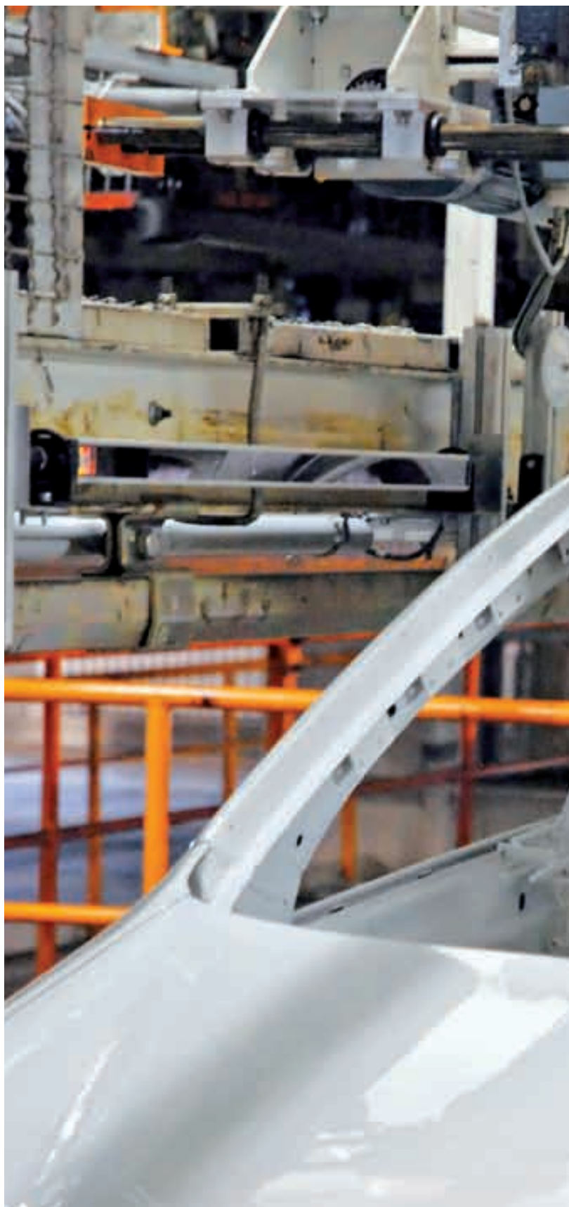
The EZ-Array measuring light curtains record the position of the car body and the grappler in real time
