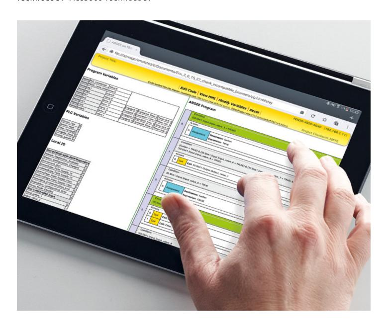
The browser-based ARGEE programming environment can also be operated with mobile devices
