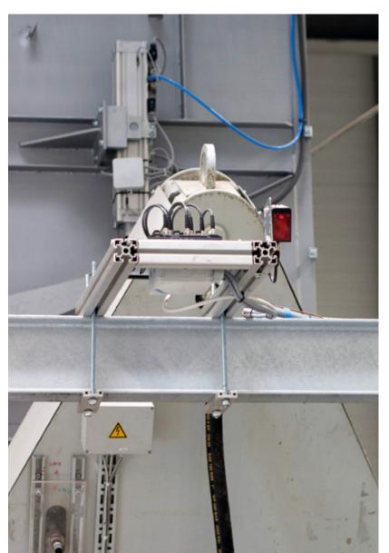
Banner's LTF12 laser sensor monitors the output of the paper bales and triggers a signal to the TBEN-S when the limit value is exceeded
